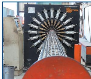
Filter Cage Fuse Welding
