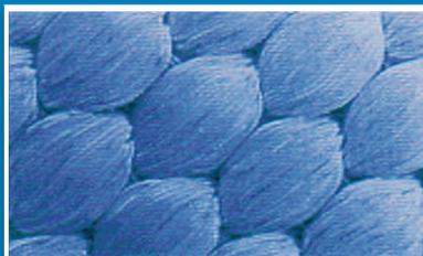
Multifilament: Consisting of several individual fibres
