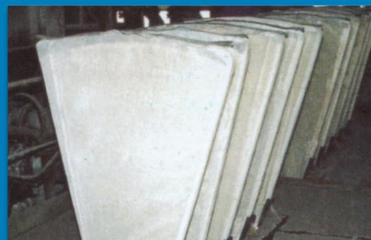
A popular choice in process filtration such as in sugar refining, fertilizer manufacturing and paper production. NFF has supplied cloths for those industries either as rolled fabrics or finished filter. With the disadvantage of high replacement and downtime cost inherent in this system, the correctness and reability of the filter media is a must.
