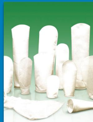
For versatile filtration systems such as High flow multi-bag pressure vessels, filter bags both in polyester & polypropylene execution are available on stock. The fabrics may be of the woven or non-woven variety while the fabric opening ranges from 1-200 microns.
