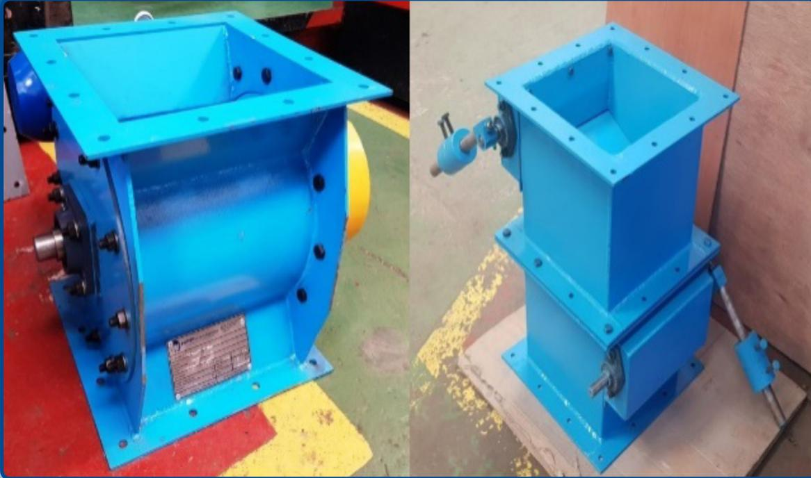
Double Flap Valve or 2-stage flap valve is a type of airlock valve commonly used in industrial application as a component in bulk material handling applications. Double Flap Valve is primarily used to discharge chunky or fibrous, bulk materials from hoppers, bin, and cyclones operating under positive or negative pressure.
